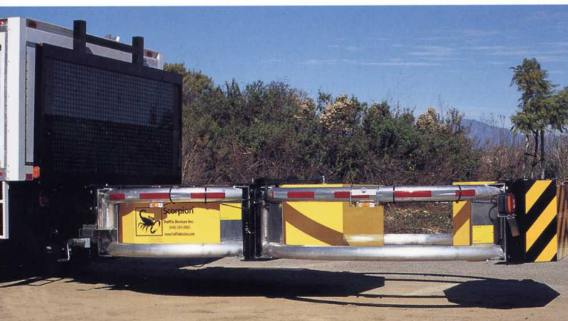
The Scorpion TMA is fully extended, with the changeable message panel in the travel or storage position.
